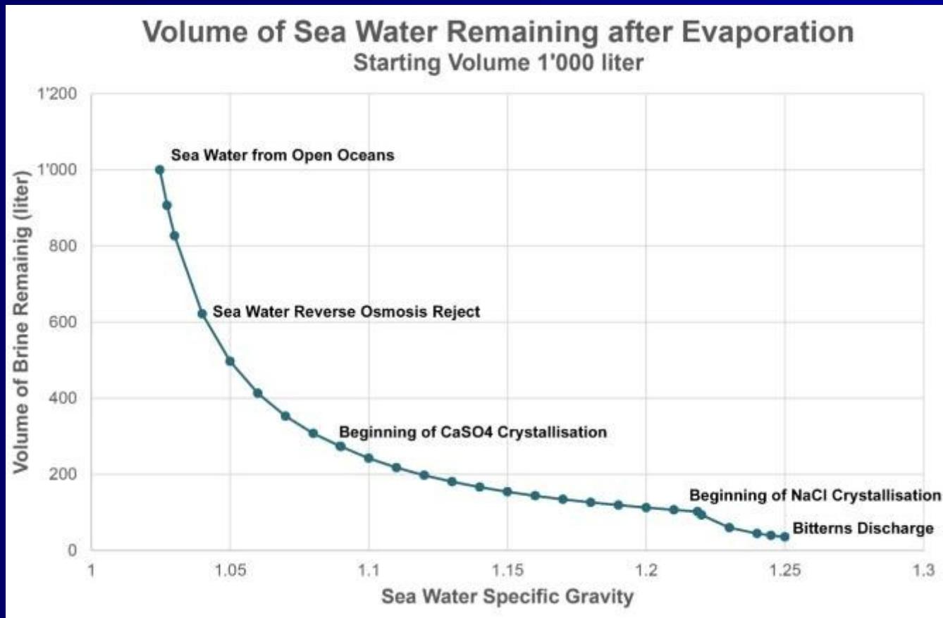
When sea water evaporates or water is being removed in a desalination process, the volume is reduced, and the concentration is rising. 96.45% of water is removed to crystallise 23.05 kg of  $\text{NaCl}$  from the original 1'000 l of sea water
