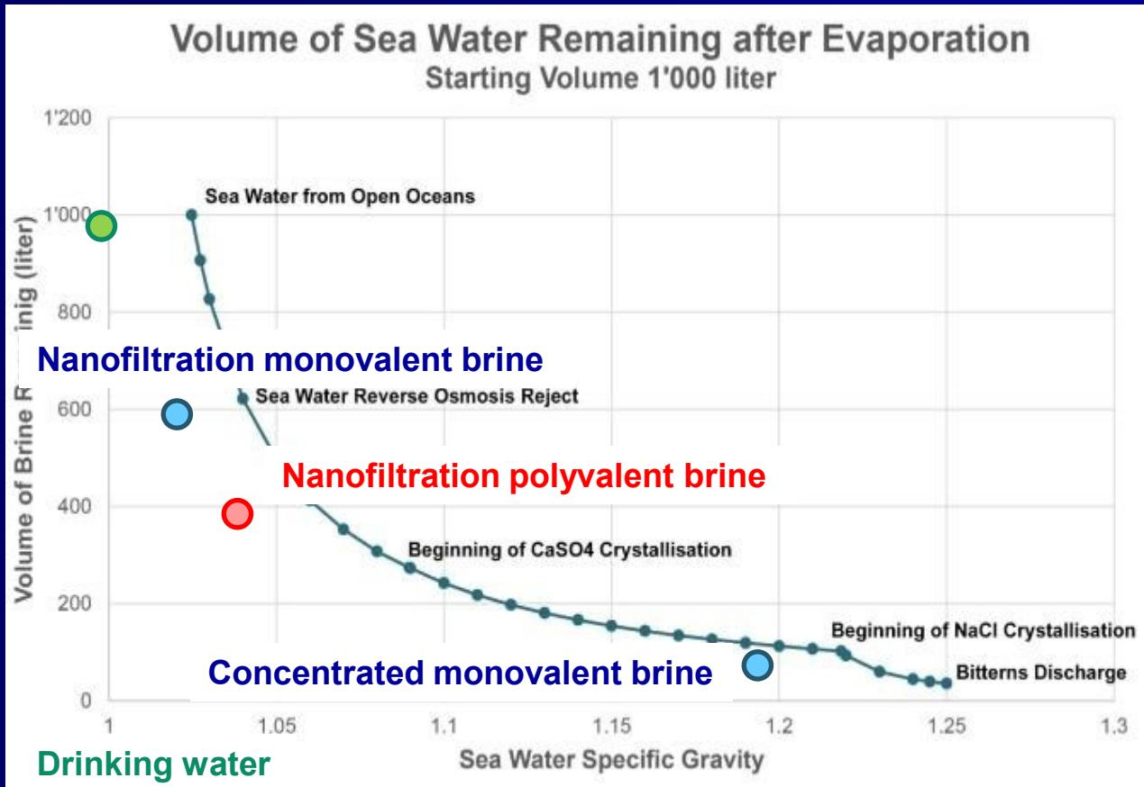
Nanofiltration splits seawater into monovalent and polyvalent streams. Water from the monovalent stream can be recovered up to 22 gpl salinity with LSRRO membranes. Rest is recovered by thermal evaporation. Water from the polyvalent stream is recovered by thermal evaporation and crystallisation. Bromine by oxidation with Cl<sub>2</sub>.
